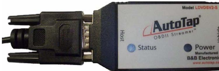
Figure D-5 OBDII Gateway with Locator cable attached
