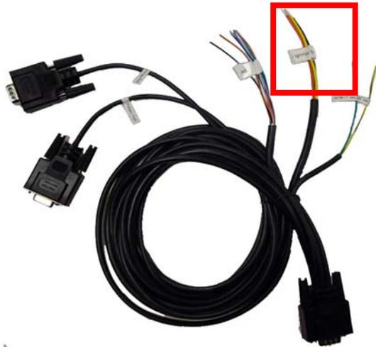
**Figure 5-1 Telemetry wires on the Locator's cable**
