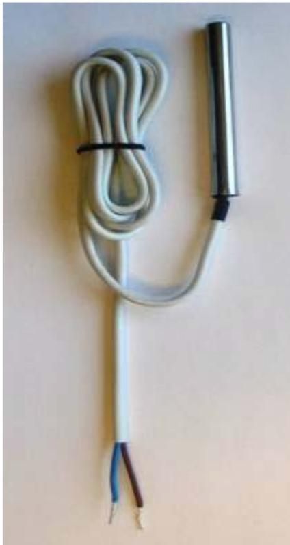
**Figure E-7** 1-wire sensor with 1M cable
